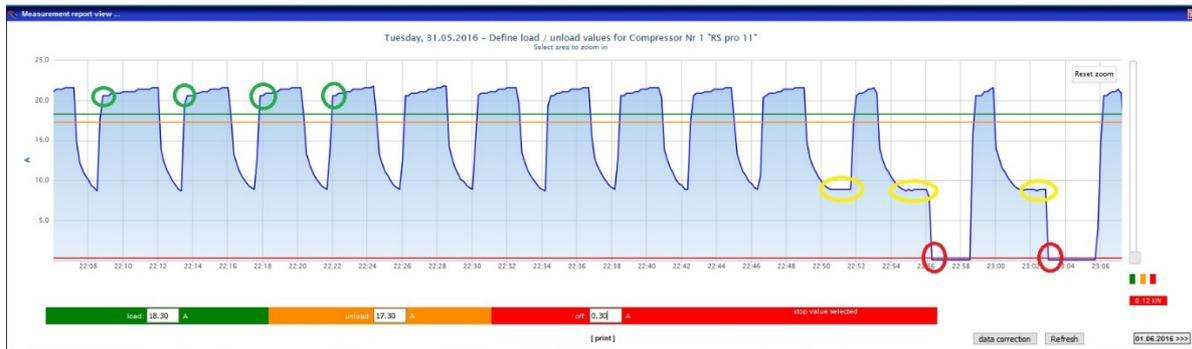
There is no maximum load line for fixed speed compressors. In this case the load/idle run line should be set between the current value at the start of the load run (here circled in green) and the fully discharged state (circled in yellow) – and certainly at a level where both the rising and the declining current curves are at their steepest.
